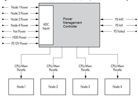
Figure 16. HP ProLiant z6000 G6 chassis node, fan, and power control block diagram
